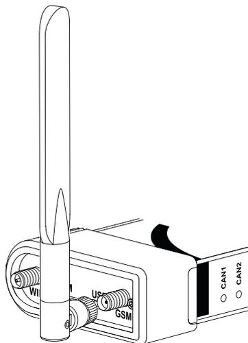
Figure 5 GSM antenna connection
