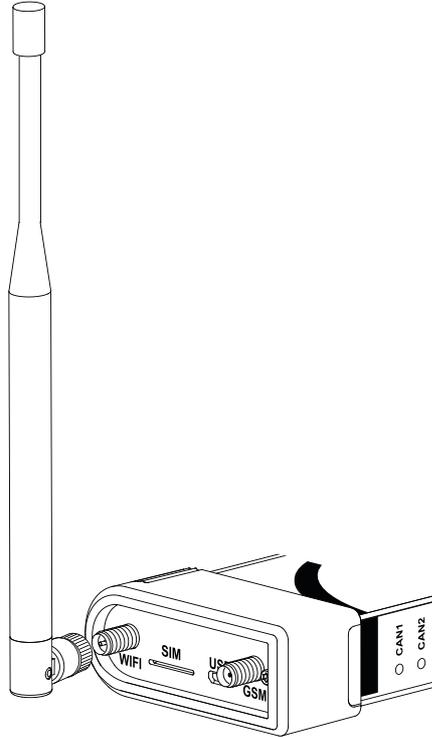
Figure 4 Wi-Fi antenna connection
