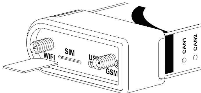
To remove the SIM card, briefly press it with a thin object until clamps click. The SIM card will partly come out of the slot, then remove it manually.
