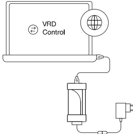
Figure 6 VRD-Client connection diagram
