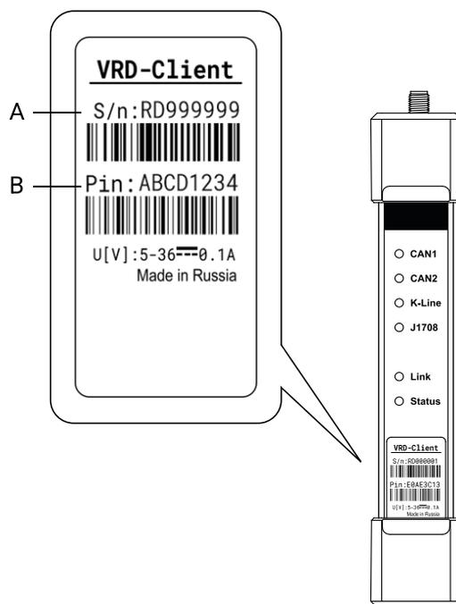
Figure 5 VRD-Client device. Serial number and pin
