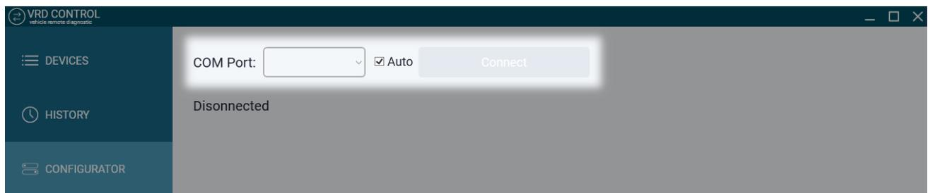
Figure 13 Automatic connection of VRD-Client to configurator
