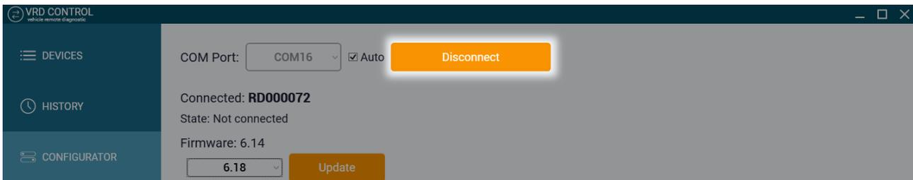
Figure 15 Disconnecting VRD-Client from configurator
